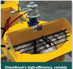
speed paddles provide reduced mix time, enhancing flow rate and
